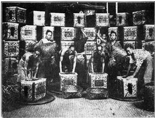
Tea being packed. The best teas are packed while still a little warm from the third and last firing
