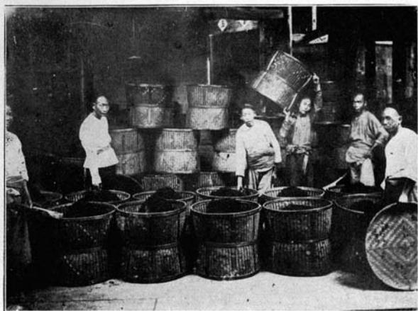
The firing process; first firing. Subsequent firings, usually two in number, are carried out in the same way.
