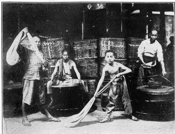
Nothing is wasted. Breaking up tea that has formed into lumps through careless manipulation. This leaf is only used for mixing in inferior grades.
