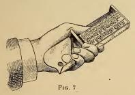
types one after another, thus forming the words of the copy before him. A space is placed after each word, to separate it from the next. The types are placed in this way, side by side, until the end of the measure is reached. Fig. 7 shows a
